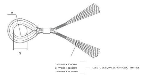
Wire Rope Ø8mm, 6 X 19 Fc galvanised ends tapered and fused or secured with rubber heat shrink.
